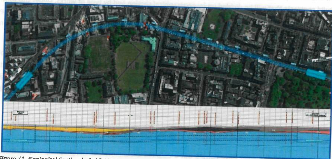
Figure 11. Geological Section (ref. A5.13, Diagram 3.13: Geologic Profile for TBM Drive C8- Tara Station to St Stephen's Green)
